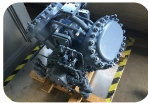
Grasso RC 49 service compressor EV0092
