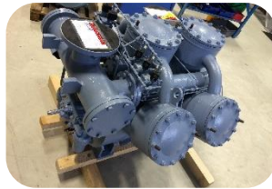
Grasso 611 service compressor EV0070
