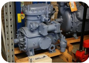
Grasso RC 29 service compressor EV
